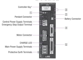
\* Make sure the linear slide model name on the controller key matches the model name of the connected linear slide. If the names do not match, the linear slide cannot be operated as specified.
