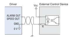
Speed output: Output at a rate of 12 pulses per motor rotation.
