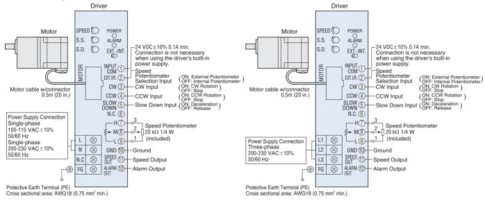
• Motor cable should be no more than 10.5 m (34.4 ft.) in length. The motor comes with 0.5m (20 in.) long connector-equipped cable which can be extended by using an accessory extension cable (sold separately).
