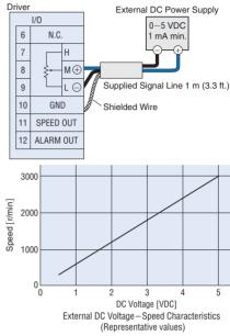
Do not allow the voltage to exceed 5 VDC, and connect the positive and negative terminals of the power supply correctly.
