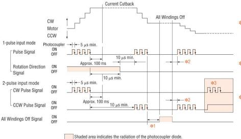
Note: 10 μs or more is the standard interval time for switching from CW to CCW. Note that the interval time varies greatly depending on the motor and load inertia.
