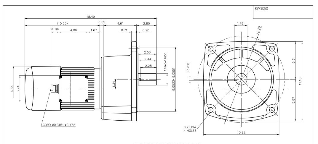
NOTE: THE RATING OF ENCLOSURE CLASS: IP65 (EN60034-5) EQUIVALENT.
