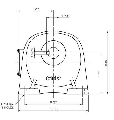
NOTE: THE RATING OF ENCLOSURE CLASS: IP65 (EN60034-5) EQUIVALENT.
