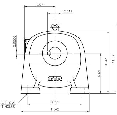
NOTE: THE RATING OF ENCLOSURE CLASS: IP65 (EN60034-5) EQUIVALENT.
