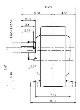
NOTE: THE RATING OF ENCLOSURE CLASS: IP65 (EN60034-5) EQUIVALENT.
