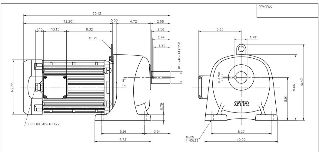
NOTE: THE RATING OF ENCLOSURE CLASS: IP65 (EN60034-5) EQUIVALENT.
