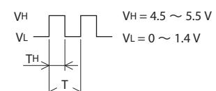
$$\text{PWM duty cycle (\%)} = \frac{T_H}{T} \times 100$$
