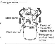
Assemble the gearhead to the motor in a condition where the motor output shaft is in an upward direction.
