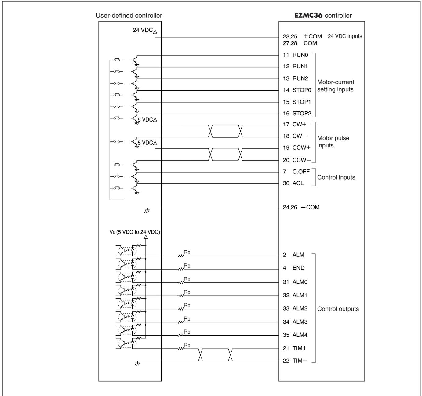
Connect the home-position detection sensors to the user-defined controller.
