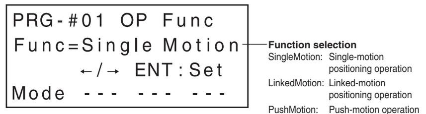
To start a positioning operation, select the number in which the operation data you wish to execute is set, using the input M0 to M5. If a number between 01 and 63 is selected, it means either the single-motion positioning operation or linked-motion positioning operation has been selected.
