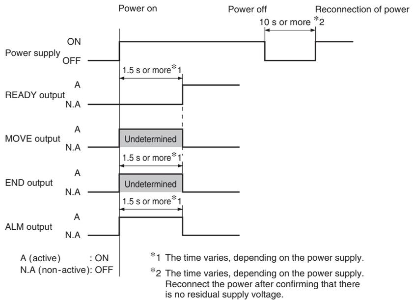
■ Figure 5-3 Output Statuses at Power-On (driver mode)
