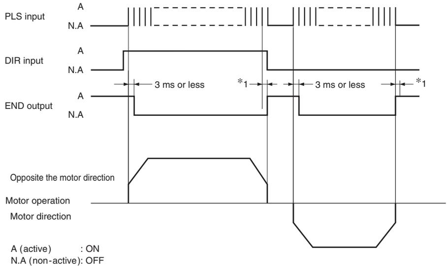
\*1 The time after the pulse train input ends until the END output becomes active varies, depending on the load and operating speed.
