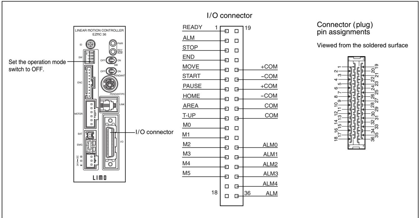
■ **Figure 4-43 Example of Standard I/O Wiring for EZMC36 Controller (driver mode)**
