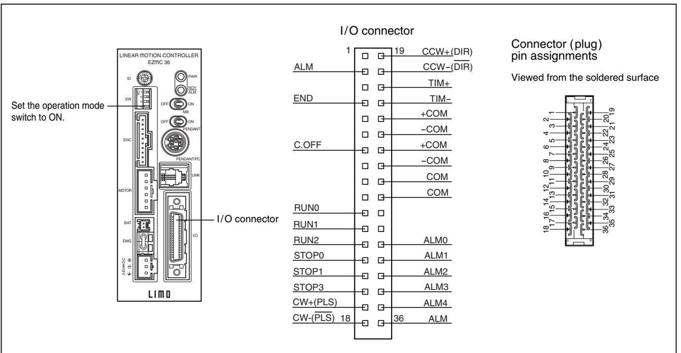
■ Figure 4-44 Example of User-Defined Controller Connection (controller mode)
