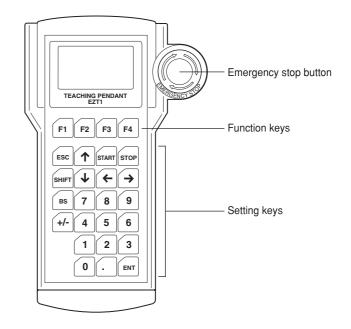
The teaching pendant has 22 setting keys and four function keys. The functions assigned to the function keys vary according to the screen.
