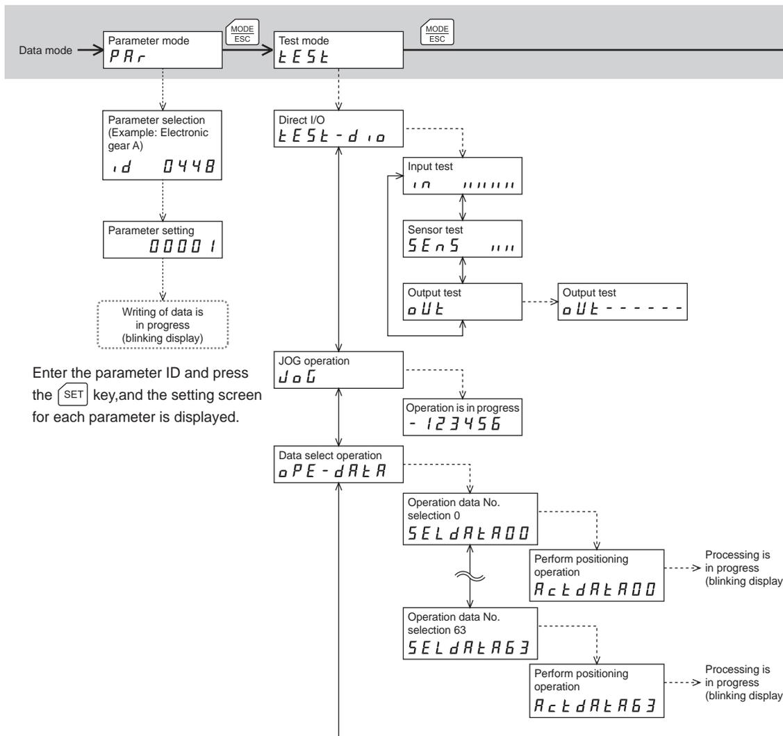
Enter the parameter ID and press the **SET** key, and the setting screen for each parameter is displayed.
