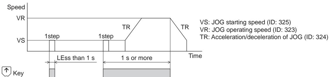
**Note** In JOG operation, the actuator operates at the set operating speed while the applicable key is pressed. Before executing JOG operation, consider the status of the equipment and condition of its surroundings to confirm thoroughly that actuator operation will not cause any dangerous situation.
