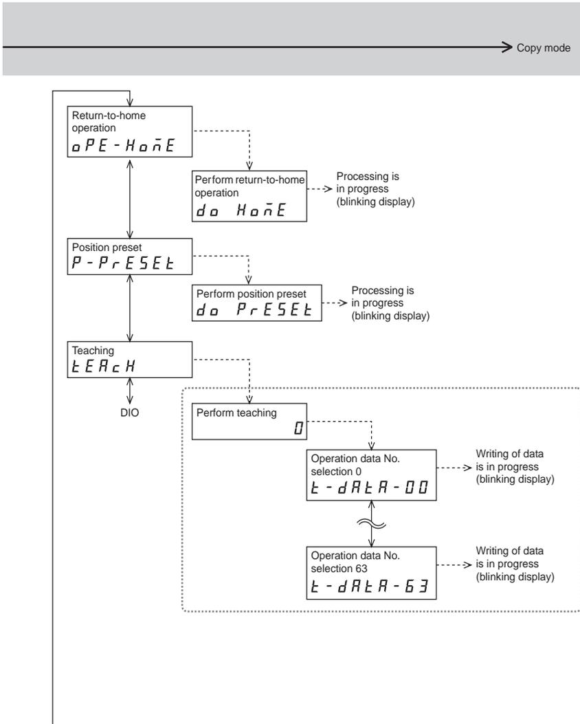
While internal processing is in progress via RS-485 communication, the process in dotted frames cannot be executed.
