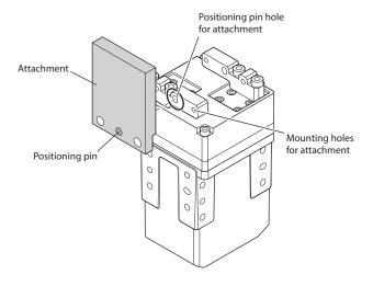
3. Secure the mounting holes for attachment with screws (not included) while pressing the attachment to the finger.
