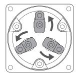
3. The moving parts (fingers) reverse, and stop after moving according to the value set in the "(HOME) Backward steps after first entry in push-homeseeking." (Factory setting: 0)
