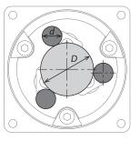
D: Outer diameter (or inner diameter) of the gripped object [mm] d: Diameter of attachment [mm]
