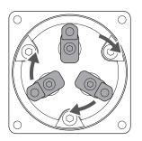
4. The moving parts (fingers) reverse again, and press against to turn the TLC output ON.
