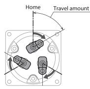
• Setting with the relative position Set the travel amount of the moving part (finger) with reference to the present position.
