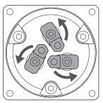
And the moving parts (fingers) move according to the value set in the "(HOME) Position offset" and stop. (Factory setting: 0)
