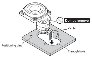
2. Move the actuator to the through hole which diameter is larger, and secure the mounting holes with screws (four pieces).
