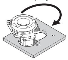
3. Secure the mounting holes with screws (four pieces).
