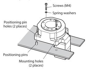
When the positioning pin holes are used as mounting holes
