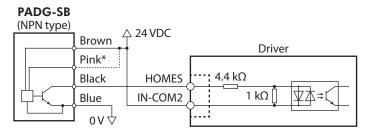
\* The logic of the sensor varies depending on the connection method. When the pink color lead is connected to the brown color lead, the sensor logic will be "normally closed."
