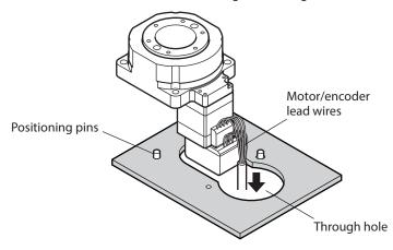
2. Move the actuator to the through hole which diameter is larger, and secure the actuator with screws.
