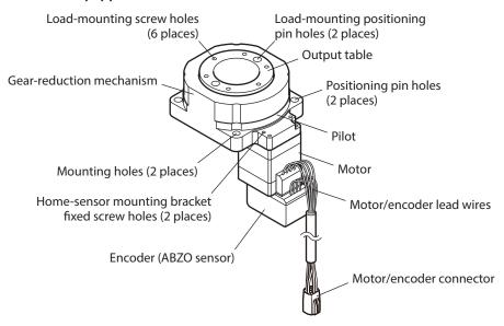
• Actuators equipped with the AR Series
