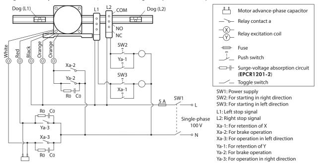
\* The contact capacity of each relay and switch must be single-phase 100 V/5 A or more, or single-phase 250 V/5 A or more.
