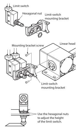
Remove the cover screw from the limit-switch mounting bracket, insert the cover onto the limit-switch mounting bracket, and then tighten the cover screw.
