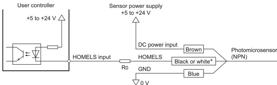
\* Connect the white lead wire when detecting the sensor output signal in normally open, and the black lead wire when detecting in normally closed.
