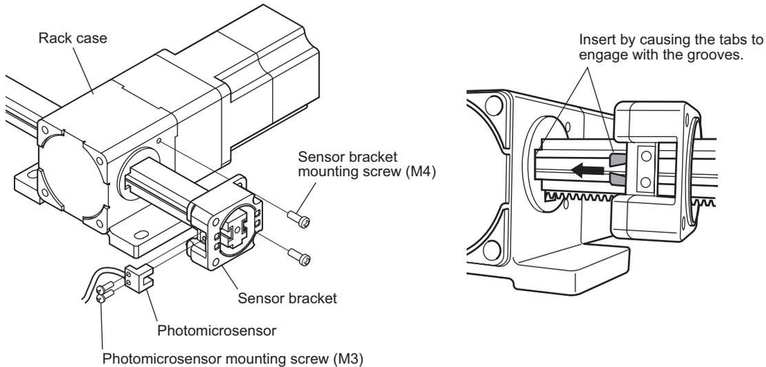
3. Connect the lead wires of the photomicrosensor to the programmable controller, etc.
