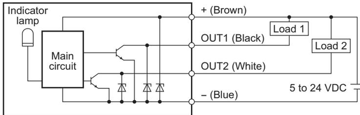
Use a power supply for a voltage of 5 VDC to 24 VDC. Also, the current should be 50 mA or less. If the current exceeds 50 mA, connect an external resistor  $R_0$ .
