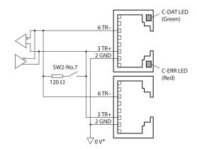
\* The GND line is used in common with the main power supply input terminal (CN1) and control power supply input terminal (TB1) [not insulated].
