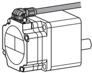
Cable outlet in opposite to output shaft direction
