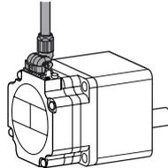
**Note** Do not apply a strong force on the locking lever of the connector for motor connection. Applying a strong force on the locking lever may cause damage.
