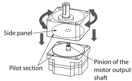
Assemble the gearhead to the motor in a condition where the motor output shaft is in an upward direction.
