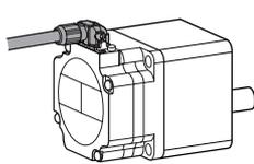
Cable outlet in vertical direction
