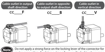
Do not apply a strong force on the locking lever of the connector for motor connection. Applying a strong force on the locking lever may cause damage.
