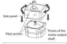
Assemble the gearhead to the motor in a condition where the motor output shaft is in an upward direction.
