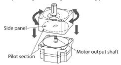
Assemble the gearhead to the motor in a condition where the motor output shaft is in an upward direction.
