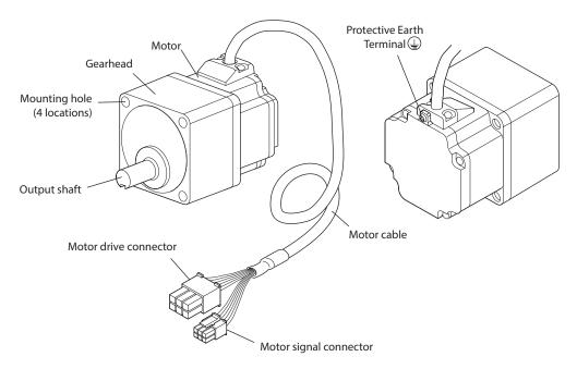
\* Illustration shows pinion shaft type/parallel shaft gearhead.
