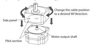
Assemble the gearhead to the motor in a condition where the motor output shaft is in an upward direction.
