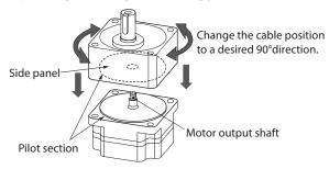
Assemble the gearhead to the motor in a condition where the motor output shaft is in an upward direction.
