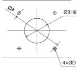
• Using the rear face as the mounting surface
