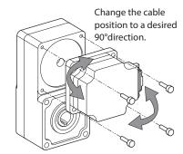
2. Check that there is no gap between the motor and the gearhead, and tighten them using the hexagonal socket head screws (4 places) included with the gearhead.
