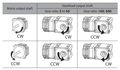
When viewing from the opposite side of the gearhead flange side, the gearhead output shaft rotates in the opposite direction to the above figure.
