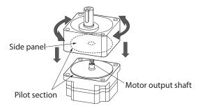
Assemble the gearhead to the motor in a condition where the motor output shaft is set upward.
