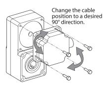
2. Check that there is no gap between the motor and the gearhead, and tighten them with hexagonal socket head screws (4 places).
