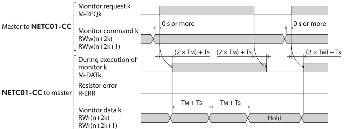
$T_M$ : Communication time between the CC-Link communication master station and remote device station (NETC01-CC) [Check the operating manual of the master station.]
