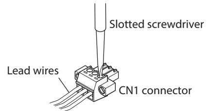
3. Insert the CN1 connector into power supply connector (CN1) and tighten the screws using a slotted screwdriver.
