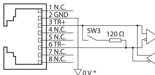
\* The GND line is used in common with CN1 (not insulated).
