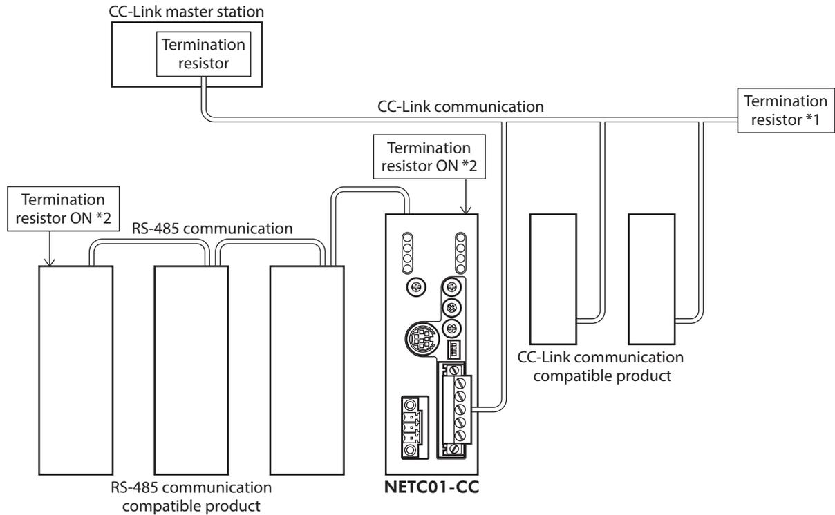
\*1 Termination resistor for CC-Link communication is not included. Use a termination resistor included with the master station.
