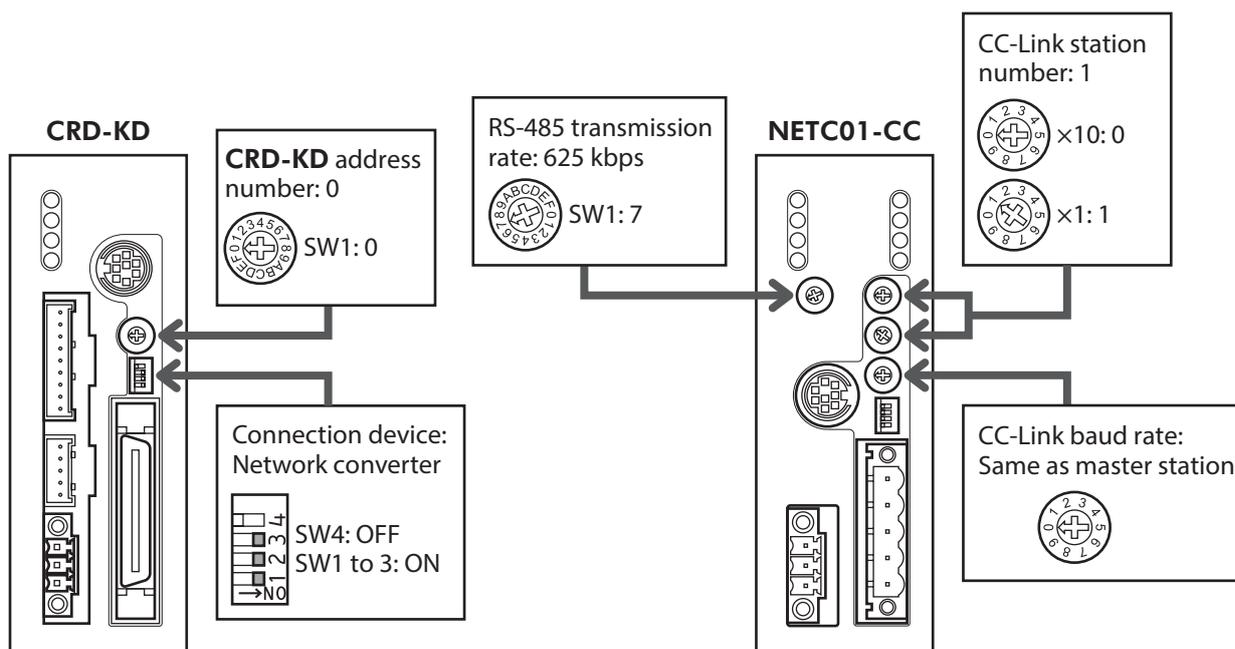
**STEP 2 Check the connection and termination resistor**
