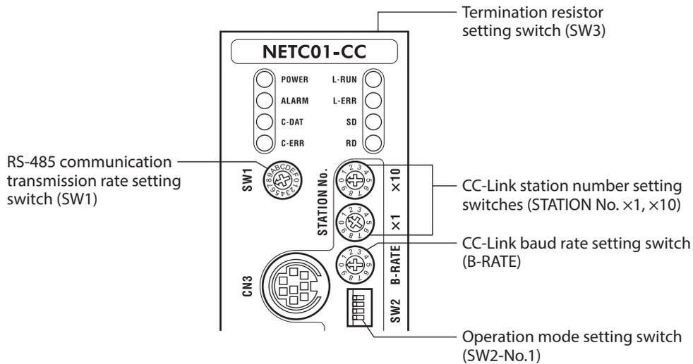
**Note** Be sure to turn off the **NETC01-CC** power before setting the switches. If the switches are set while the power is still on, the new switch settings will not become effective until the **NETC01-CC** power is cycled.
