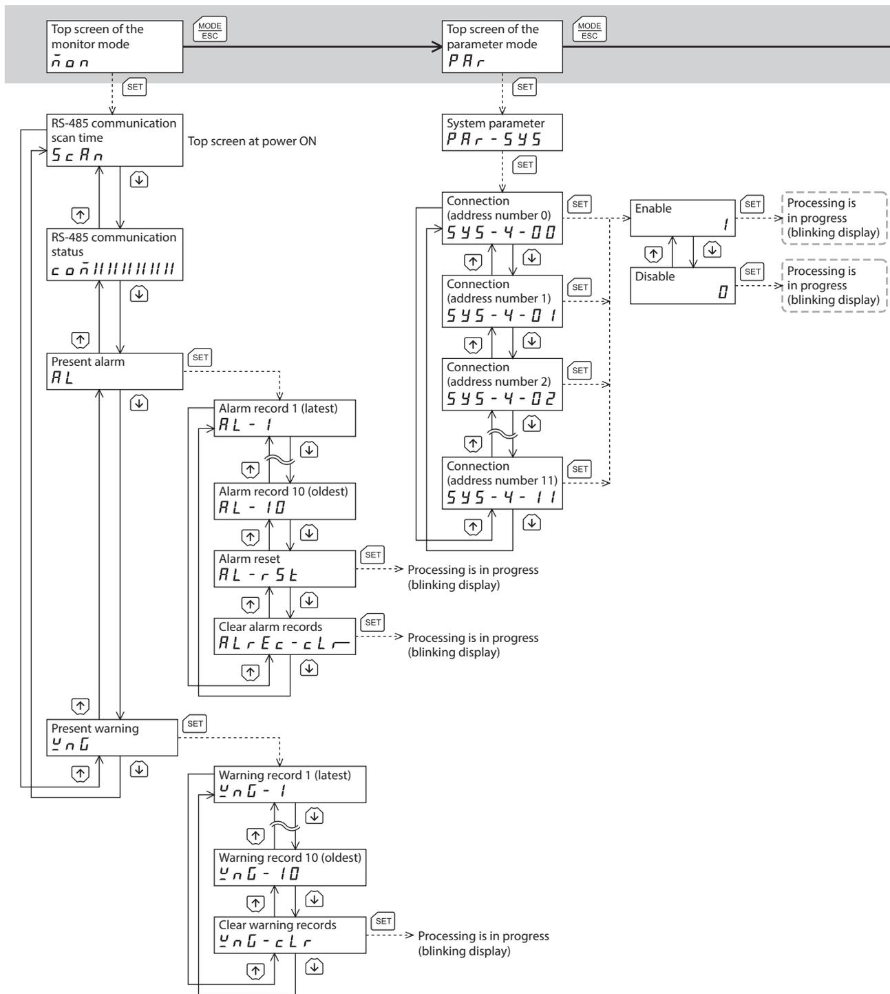
In the lower level except the top screen, press the **MODE ESC** key to return to the previous level.
