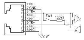
\* The GND line is used in common with CN1 (not insulated).
