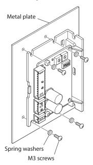
$\bullet$  When using the cutouts for mounting B
