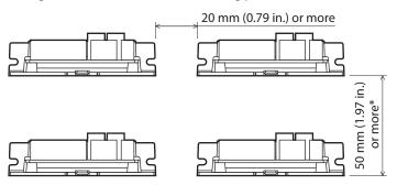
$<sup>^{\</sup>ast}$  Provide 40 mm (1.57 in.) clearances for the "driver with mounting plate" of Type A.
