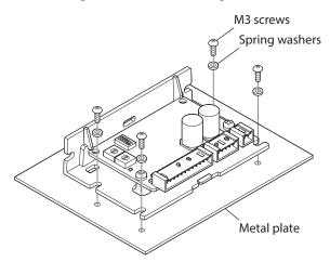
• When using the cutouts for mounting B
