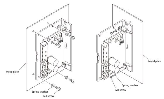
Install the driver using either of the "cutout for mounting A" or "cutout for mounting B." Do not concurrently use both cutouts.
