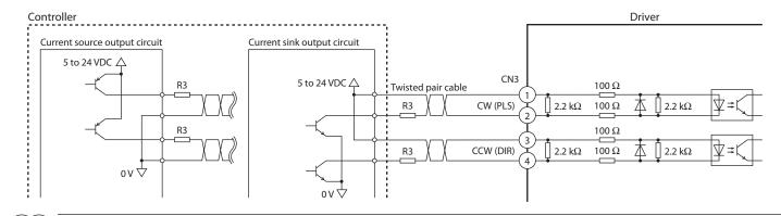
Use the CW input and CCW input at 5 VDC. If the voltage exceeding 5 VDC is applied, connect an external resistor R3 so that the input current becomes 7 to 20 mA.
