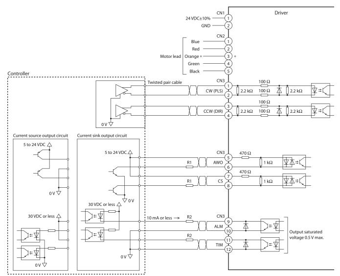
\* This orange lead wire is for 5-phase stepping motor. For 2-phase stepping motor, do not connect anything to the pin No.3 since there is no orange lead wire.
