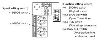
Two different operating speeds of high speed and low speed can be set in the driver.
