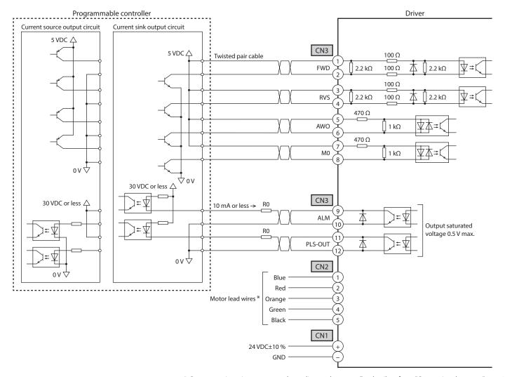
${}^*\ Connector\ pin\ assignments\ vary\ depending\ on\ the\ motor.\ For\ details, refer\ to\ "Connecting\ the\ motor"\ on\ p.6$
