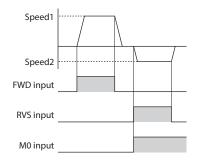
Two setting patterns are available for the Speed1 and Speed2, and they vary depending on the setting of the SPD2 EN switch (function setting switch No.2).
