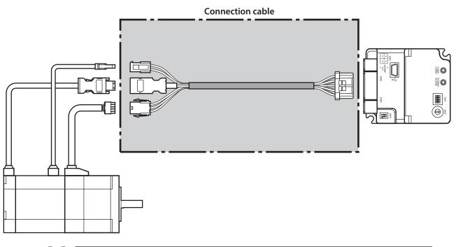
$(\mathsf{memo})$  When installing the motor on a moving part, use a flexible cable.
