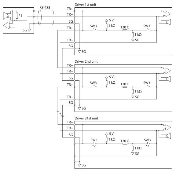
\*1 Termination resistor 120  $\Omega$
