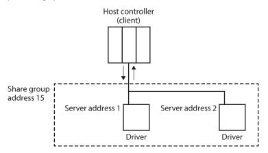
When a query is sent from the client to the share group address 15, the server addresses 1 and 2 start positioning operation. When each server executes the processing, a response is returned sequentially. The order in which responses are returned is set in the "Share control local ID" parameter. ( $\Box$  p.29)
