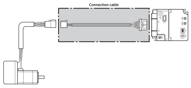
(memo) When installing the motor on a moving part, use a flexible cable.
