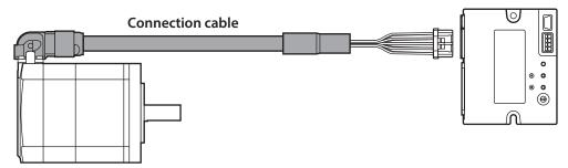
The model name of the connection cable varies depending on the outlet direction from the motor. Refer to the figures below.
