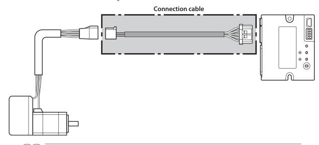
(memo) When installing the motor on a moving part, use a flexible cable.
