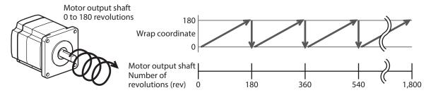
The present position of the motor is preset every 180 revolutions, however, the 32-bit counter in the driver is not preset.
