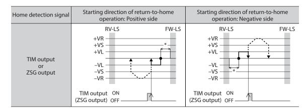
\* After pulling out of the limit sensor, the motor rotates according to the value set in the (HOME) Backward steps in 2 sensor home-seeking (4169h) and stops.
