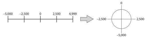
Example 2: Coordinates when the wrap setting range is 1,800 rev and the resolution is 10,000 P/R
