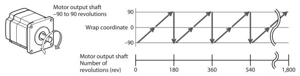
When the wrap setting range is exceeded, the sign is reversed.
