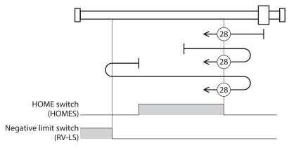
In the case of return-to-home operation of Oriental Motor's specifications, the same operation is performed if the following data is set.
