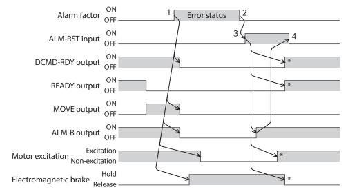
\* It is the movement when the excitation command is input from the MainDevice at the time the ALM-RST input is turned ON.
