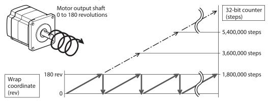
The present position of the motor is preset by 180 revolutions, however, the 32-bit counter is not preset. The value of the 32-bit counter can be checked by the Command position 32-bit counter (4091h). The 32-bit counter goes around between –2,147,483,648 and 2,147,483,647.
