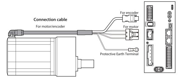
The model name of the connection cable varies depending on the outlet direction from the motor. Refer to the figures below.
