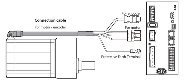
The model name of the connection cable varies depending on the outlet direction from the motor. Refer to the figures.
