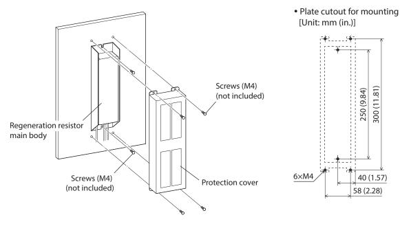
The regeneration resistor main body will reach a high temperature. Be sure to use it with the protection cover to prevent hands from touching. Failure to do so may result in a skin burn(s).
