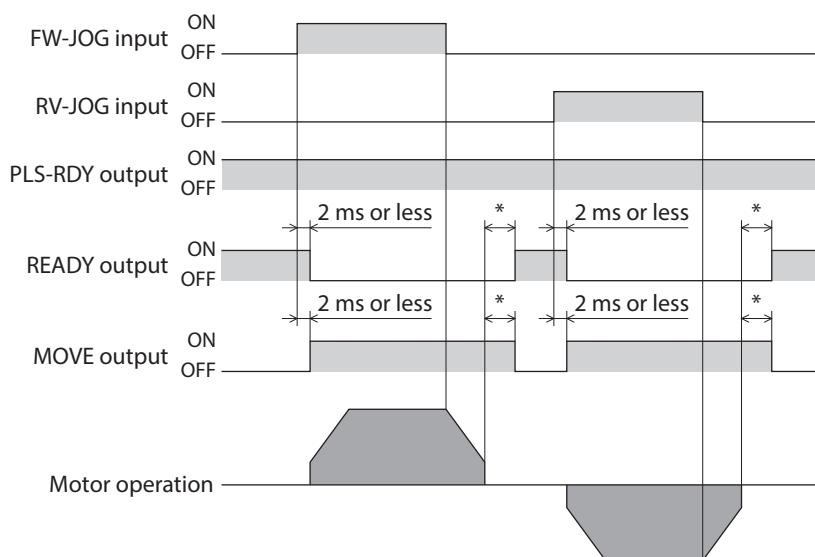
\* It varies depending on the load, operating velocity, speed filter, etc.
