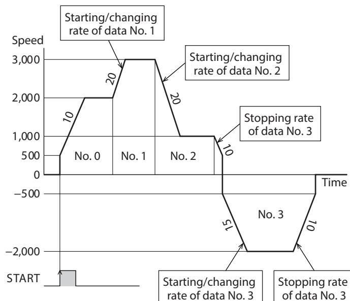
\* If the direction of operation is switched to the opposite direction in the middle of operation, the target position will be exceeded.
