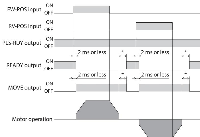
\* It varies depending on the load, operating speed, speed filter, etc.
