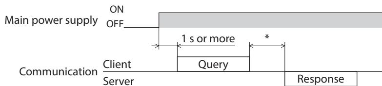
\* C3.5 (silent interval) + Tb5 (query processing time (driver)) + Tb2 (transmission waiting time (driver side))
