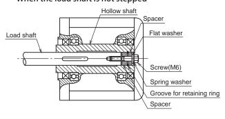
Refer to chart below for hollow shaft inside dimensions and the recommended load shaft dimensions.
