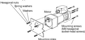
Drill holes in the mounting plate and fasten the motor to the mounting plate with the provided mounting screws, hexagonal nuts, washers and spring washers. Be sure that no gaps are left between the gearhead and the surface of the mounting.
