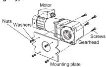
Drill holes in the mounting plate and fasten the motor to the mounting plate with screws, nuts, and washers (The mounting screws are not provided.). Be sure that no gaps are left between the motor and the surface of the mounting plate. \* Illustration shows BH6G2-□RH.
