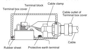
To ensure safety, ground the motor using the protective earth terminal  $\bigoplus$  inside the terminal box.
