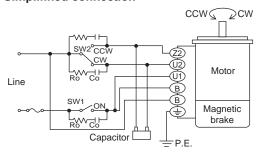
**Note** Wiring cannot be simplified for vertical drive applications or three-phase motors.
