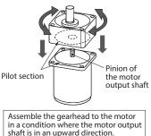
Check no gaps remain between the motor and gearhead, and tighten them with hexagonal socket head screws (2 pieces).
