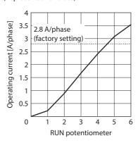
Current corresponding to a dual-phase value flows to the ammeter. A value of one-half that which is indicated equals the single-phase current value.
