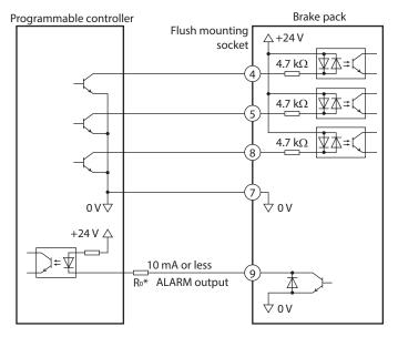
Recommended resistance value when the current-limiting resistor Ro is connected  $2.7 \text{ k}\Omega \text{ to } 4.7 \text{ k}\Omega \text{ (1 W)}$
