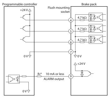
\* Recommended resistance value when the current-limiting resistor Ro is connected  $2.7 \text{ k}\Omega \text{ to } 4.7 \text{ k}\Omega \text{ (1 W)}$
