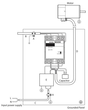
A: Cable clamp D: Motor cable [10 m (32.8 ft.)]
