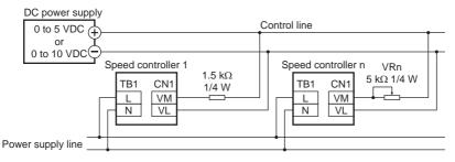
Current capacity (I) of external DC power supply when the number of speed controllers is n: Current capacity (I) =  $1 \times n \text{ (mA)}$
