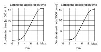
\* However, when the load inertia is large, the deceleration time cannot be set at a shorter time than how long it takes for the motor to coast to a stop.
