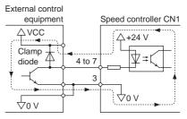
the external control equipment power. When powering up, turn on the external control equipment power first, followed by the speed controller power.
