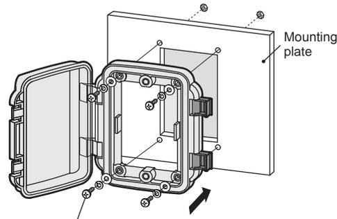
Frame thickness of screw hole 5 mm (0.20 in.)
