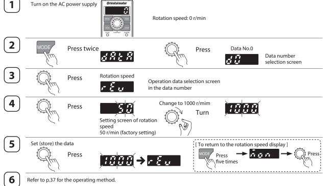
If the display is not shown as the above steps, check "Setting of operation data" of the operation panel on p.50.
