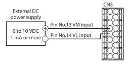
Be sure to use the external DC voltage at 10 V or lower. When connecting the external DC power supply, make sure the polarities are correct. Reversing the polarities may cause damage to the driver.
