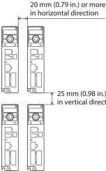
in horizontal direction 25 mm (0.98 in.) or more in vertical direction
