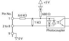
Changing the logic level setting of input signals
