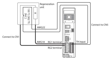
Be sure to connect the thermostat output to the TH input when using the regeneration resistor.
