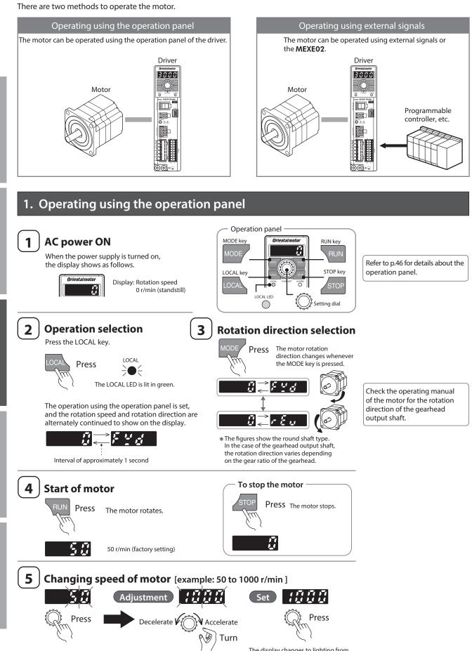
The display blinks. You can adjust the speed while blinking. The display changes to lighting from blinking, and the speed will be set. When you start the motor next time, it will rotate at the set speed.
