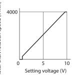
$$\frac{\text{Analog operation speed}}{\text{command gain*}} = \frac{\text{Speed upper limit}}{\text{Maximum value of setting voltage}}$$
