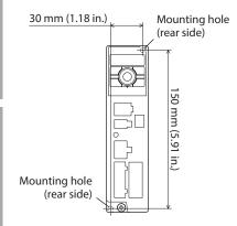
• When two or more drivers are installed When two or more drivers are installed side by side, provide 20 mm (0.79 in.) and 25 mm (0.98 in.) clearances in the horizontal and vertical directions, respectively.
