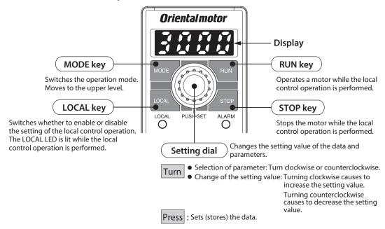
Local control operation: This is a method to operate using the operation panel. Remote control operation: This is the method to operate using the external signals or **MEXEO2**.
