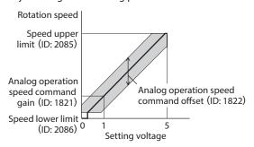
Analog operation Analog operation Analog operation = speed command × Setting voltage + speed command speed command gain
