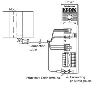
However, the grounding resistance value provided in the standards applied to the equipment may not be satisfied depending on the type or length of the connection cable.
