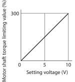
Analog torque limiting gain\* =  $\frac{\text{Analog torque limiting}}{\text{Maximum value of setting voltage}}$
