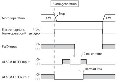
\* The electromagnetic brake will activate to hold the load at the moment an alarm generates.
