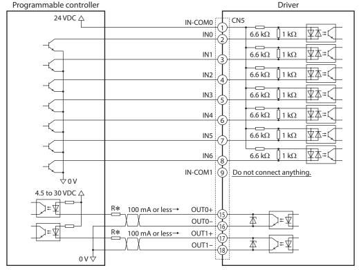
\* Recommended resistance value when the current limiting resistor R is connected In the case of 24 VDC: 680  $\Omega$  to 2.7 k $\Omega$  (2 W) In the case of 5 VDC: 150  $\Omega$  to 560  $\Omega$  (0.5 W)
