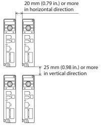
• When drivers are installed in a close contact state Install drivers to a flat metal plate offering high heat conductivity [corresponding to an aluminum plate of 350×350×2 mm (13.78x13.78x0.08 in.) or larger].
