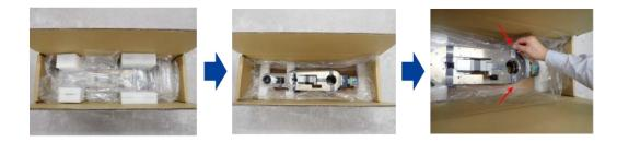
3. Take out the product holding the motor of the 1st axis (M1) and the motor of the 2nd axis (M2) with both hands.
