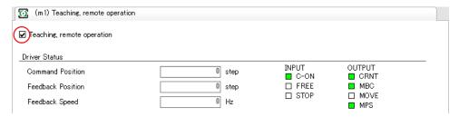
3. Use buttons on the pane to operate the motor.
