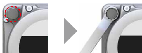
Figure 18. Shape Possible to Use Hexagon Head Bolts
