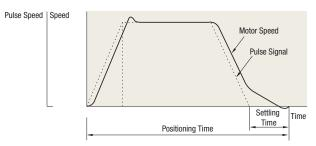
• The factory setting for settling time on the NX Series is 60~70 ms. However, the settling time varies when the gain parameter is changed by the mechanical rigidity setting switch.
