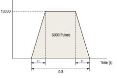
(4) Calculate the operating speed NM [r/min]
