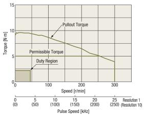
The **PS** geared type can use acceleration torque up to the maximum torque range to start and stop inertia loads.
